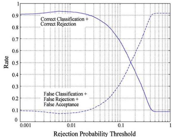
Fig. 9. Dependency of correct and false decision rates on rejection threshold.
