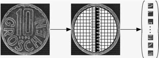
Fig. 1. Rearrangement of the inner pixels of a coin into a vector.
