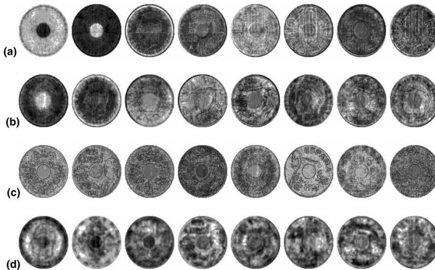
Fig. 4. First 8 eigenimages constructed from: (a) intensity images, (b) equalized intensity images, (c) edge images, (d) smoothed edge images.
